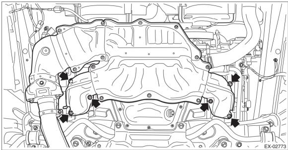
2) Install the bolts, springs, and nuts which secure the rear exhaust pipe to the center exhaust pipe. NOTE:
