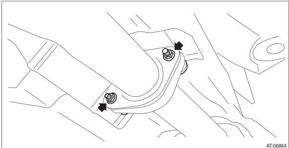
3) Tighten the bolts which secure the center exhaust pipe to the hanger bracket.
