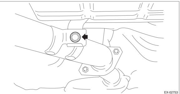
7) Remove the front exhaust pipe and center exhaust pipe from vehicle as a unit.
